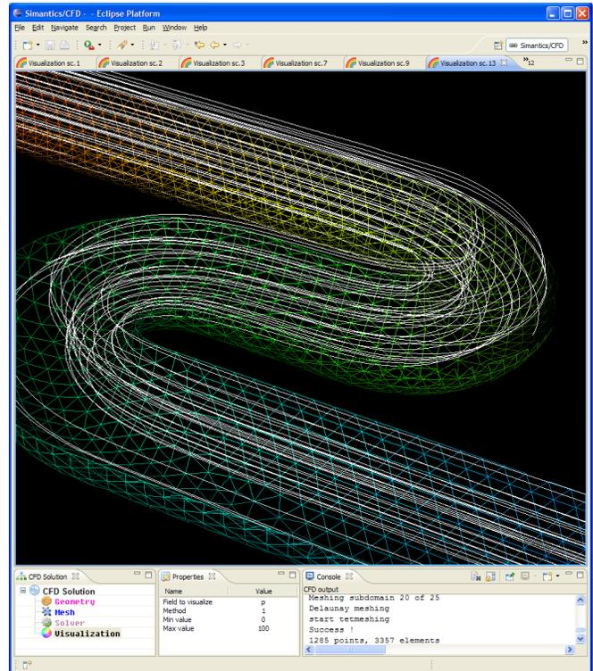
Figure 7. Stream lines visualization in a pipe.
