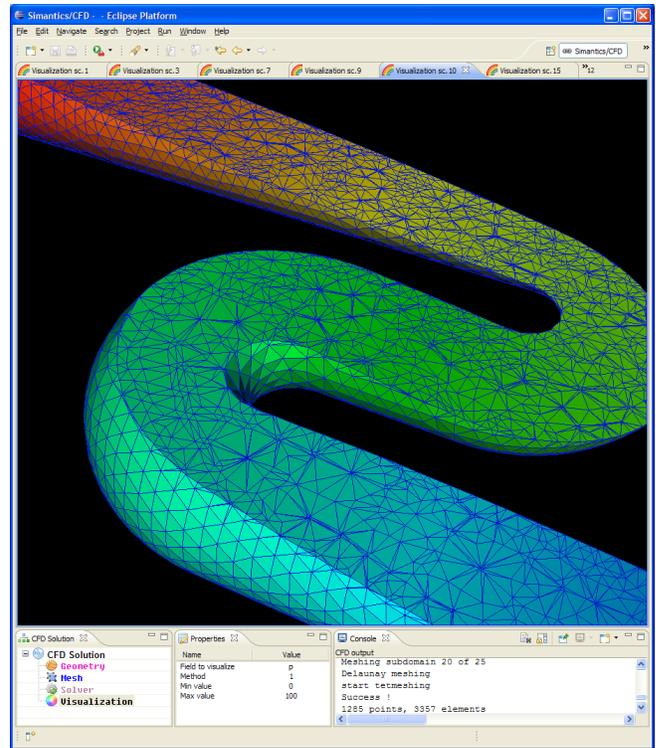
Figure 6. 3D cut plot visualization of pressures inside a pipe.
