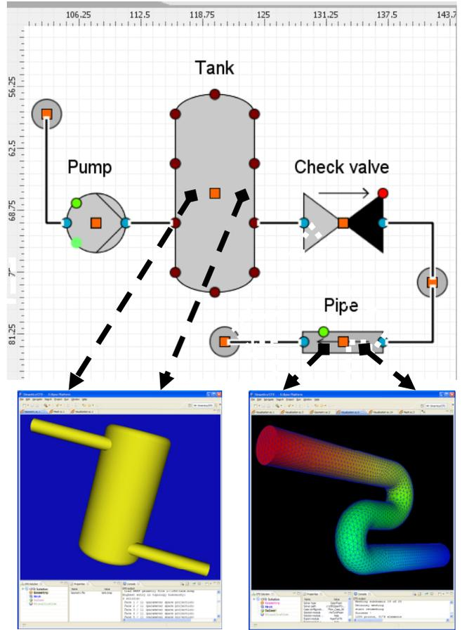
**Figure 2.** Illustrative schema of the link between 1D process simulator (Apros 6) and the 3D CFD model perspective.
