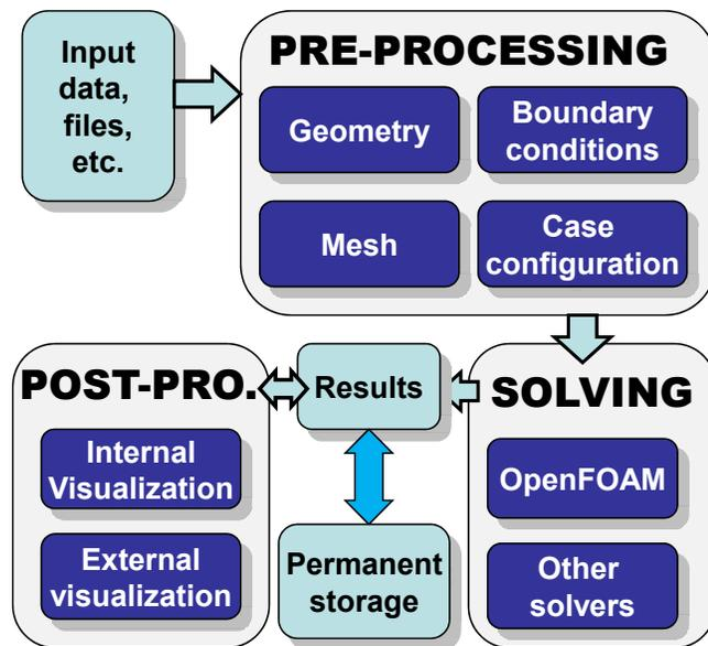
Figure 3. A schema of CFD modelling workflow and components used in our approach.
